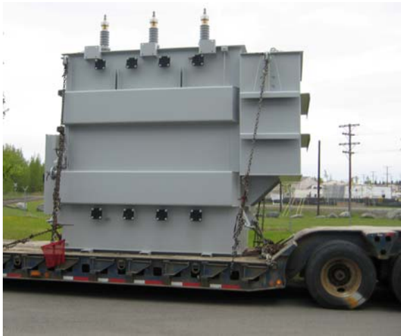
Transport of transformer for the substation
